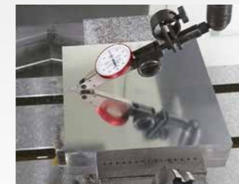
DYPEC ® mirror milling with ball end mill
