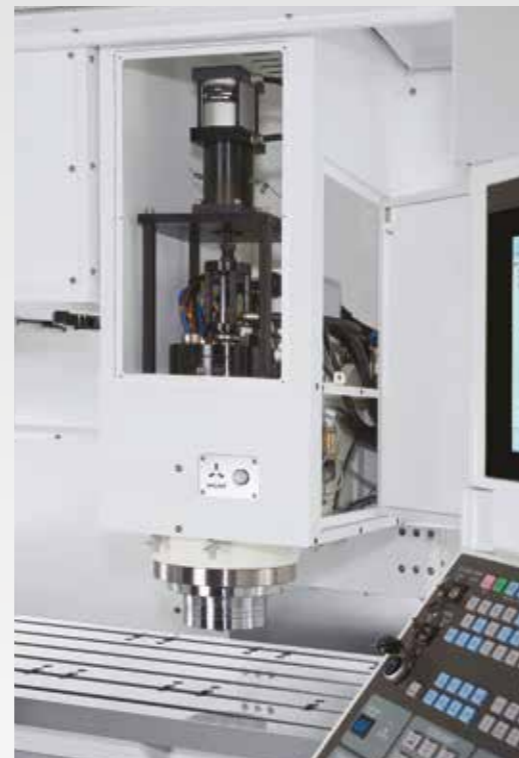
Headstock service door to facilitate access is standard on all models.
