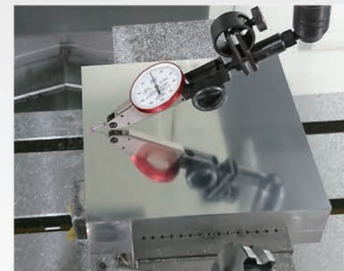
DYPEC ® mirror milling with ball end mill
